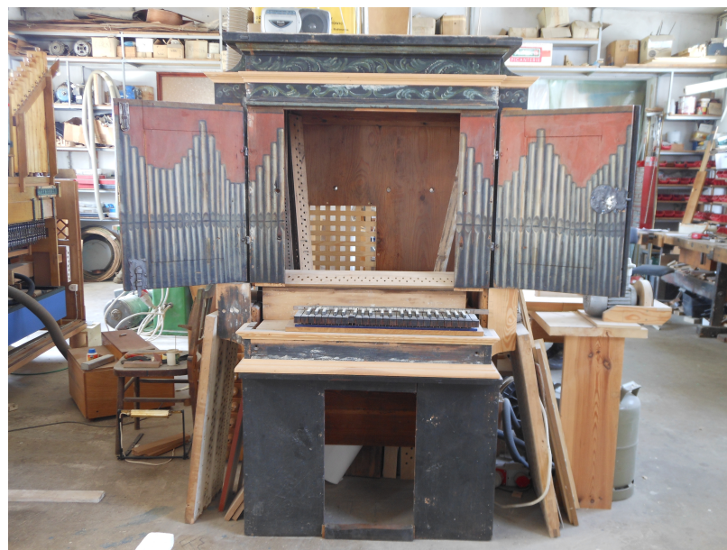
Figure 1. Open chest organ (pipes depicted on the door).
